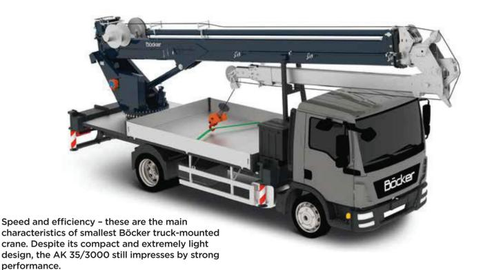
With an extension length of 35 m and a working range up to 26.6 m, this crane reaches impressive working radiuses. The fly jib us mechanically extendible up to 11.2 m so that the working area can be optimally used.
